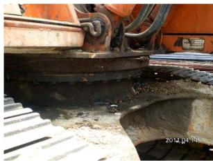
Too much lubricant grease was observed on the plant, the Contractor should clean up excess grease to avoid any contamination to soil.
