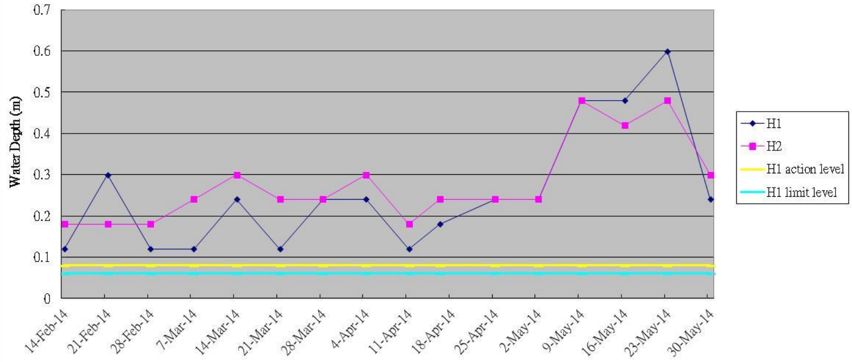
Graphical plots of Hydrological Monitoring(water depth at ebb tide) for H1 & H2
