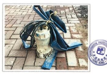
CNP 283 Water pump, submersible (electric) 潛水泵 (電動)
