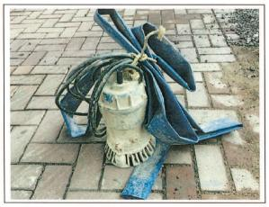
CNP 283 Water pump, submersible (electric) 潛水泵 (電動)
