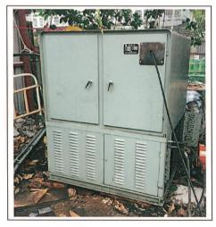
Power pack (diesel) 油渣動力供應器
