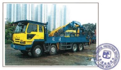
Lorry with crane, 5.5 tonne<gross vehicle weight≦38 tonne 吊臂貨車,5.5 噸<總重量≦38 噸
