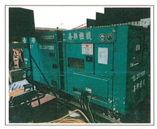
Generator, with Quality Powered Mechanical Equipment Label showing a Sound Power Level ≦94dB(A) 發電機,備有優質機動設備標籤顯示聲功率級≦94 分貝(A)
