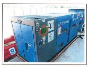
Generator, with Quality Powered Mechanical Equipment Label showing a Sound Power Level ≦93 dB(A) 發電機,備有優質機動設備標籤顯示聲功率級≦93 分貝(A)
