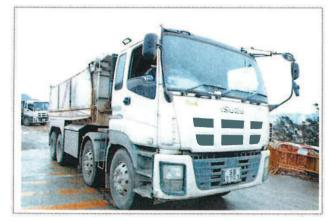
Dump truck, 5.5 tonne<gross vehicle weight≦38 tonne 卸土車, 5.5 噸<總重量≦38 噸
