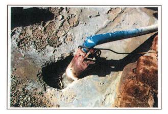
CNP 283 Water pump, submersible (electric) 潛水泵 (電動)
