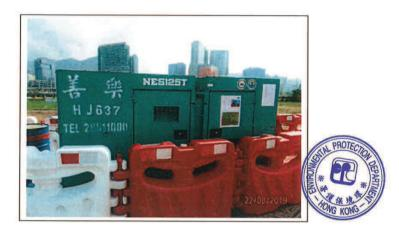
Generator, with Quality Powered Mechanical Equipment Label showing a Sound Power Level ≦93 dB(A) 發電機,備有優質機動設備標籤顯示聲功率級≦93 分貝(A)
