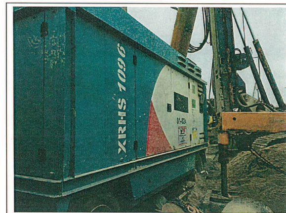
Air compressor, with Noise Emission Label showing a Sound Power Level of \leq 104\text{dB(A)} (2) 空氣壓縮機，備有噪音標籤顯示聲功率級 \leq 104 分貝(A) (二)
