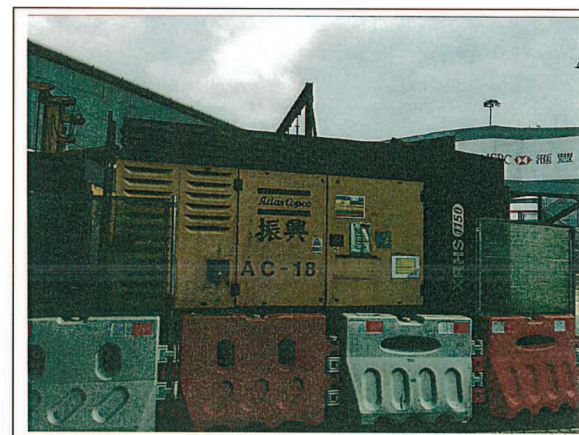
Air compressor, with Noise Emission Label showing a Sound Power Level of \leq 104\text{dB(A)} (1) 空氣壓縮機，備有噪音標籤顯示聲功率級 \leq 104 分貝(A) (一)
