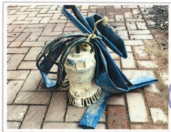
CNP 283 Water pump, submersible (electric)
