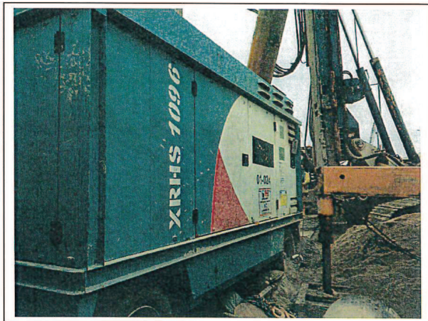
Air compressor, with Noise Emission Label showing a Sound Power Level of \leq 104\text{dB(A)} (2)
