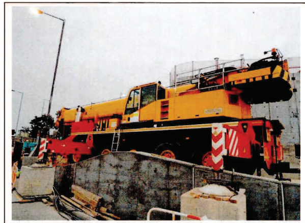
CNP 048 Crane, mobile (diesel) 起重機，流動 (油渣)
