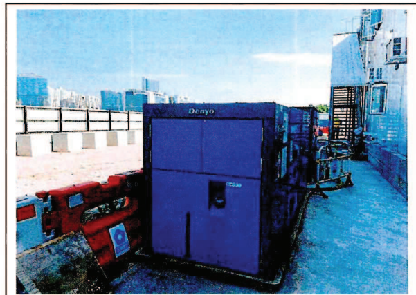
Generator, with Quality Powered Mechanical Equipment Label showing a Sound Power Level \leq 93 dB(A) (2) 發電機，備有優質機動設備標籤顯示聲功率級 \leq 93 分貝(A) (二)
