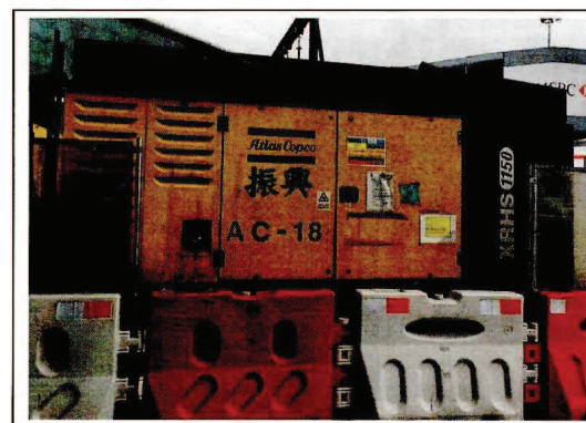
Air compressor, with Noise Emission Label showing a Sound Power Level of \leq 104 dB(A) 空氣壓縮機，備有噪音標籤顯示聲功率級 \leq 104 分貝(A)
