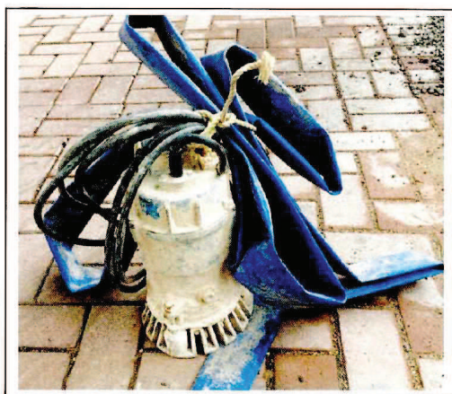
CNP 283 Water pump, submersible (electric) 潛水泵 (電動)
