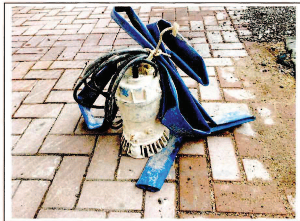
CNP 283 Water pump, submersible (electric) 潛水泵 (電動)
