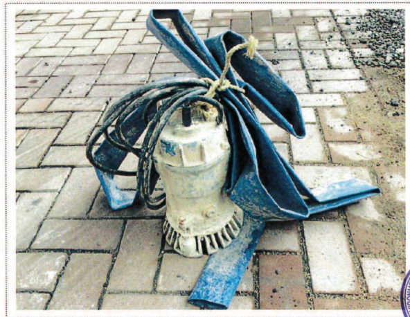
CNP 283 Water pump, submersible (electric) 潛水泵 (電動)
