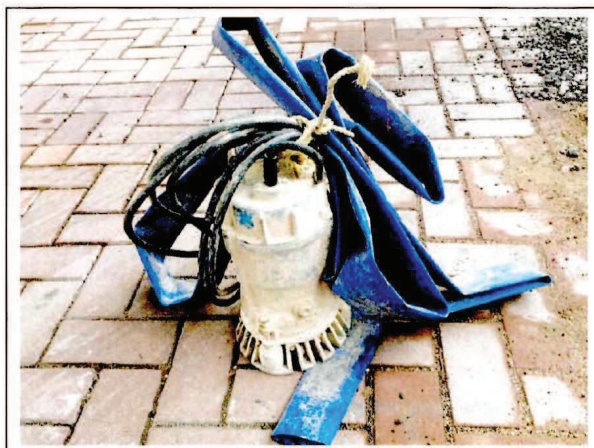
CNP 283 Water pump, submersible (electric) 潛水泵 (電動)
