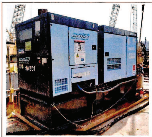
Generator, with Quality Powered Mechanical Equipment Label showing a Sound Power Level \leq 95 dB(A) 發電機，備有優質機動設備標籤顯示聲功率級 \leq 95 分貝(A)
