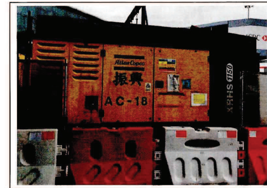
Air compressor, with Noise Emission Label showing a Sound Power Level of \leq 104 dB(A)
