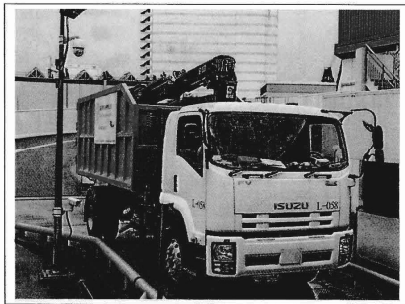
Dump truck, with grab, 5.5 tonne<gross vehicle weight≤38 tonne 抓斗卸土車，5.5噸<總重量 ≤38噸
