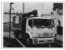
Dump truck, with grab, 5.5 tonne<gross vehicle weight  $\leq$  38 tonne 抓斗卸土車,5.5 噸<總重量  $\leq$  38 噸
