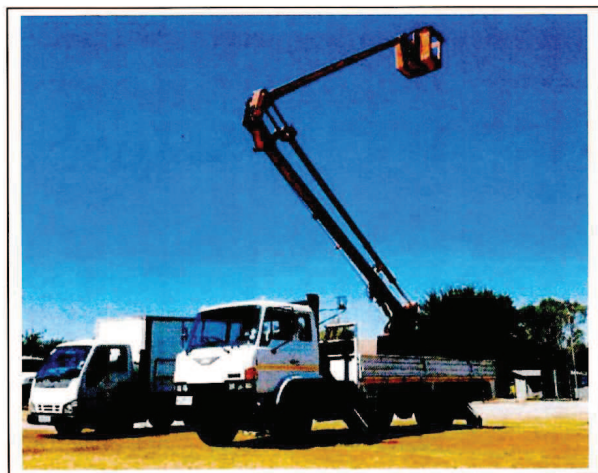
Lorry, with aerial platform, 5.5 tonne < gross vehicle weight \leq 38 tonne 升降台貨車，5.5噸 < 總重量 \leq 38噸
