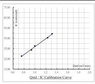
$Calibration \ curve \ requirements: \quad (A). \ \ r > 0.990 \ ; \ \ (B). \ \ At \ least \ 3 \ Qstd \ numbers \ are in the \ TSP \ range \ (\ 1.1 - 1.7 \ m3 \ / \ min \ ).$
