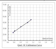
Calibration curve requirements : (A). r > 0.990; (B). At least 3 Qstd numbers are in the TSP range (1.1 - 1.7 m3 / min).
