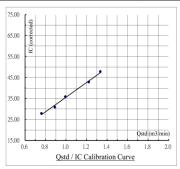
Calibration curve requirements : (A). r > 0.990; (B). At least 3 Qstd numbers are in the TSP range (1.1 - 1.7 m3 / min).
