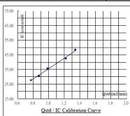
$Calibration \ curve \ requirements: \quad (A). \ \ r > 0.990 \ ; \quad (B). \ \ At \ least \ 3 \ Qstd \ numbers \ are \ in \ the \ TSP \ range \ (\ 1.1 - 1.7 \ m3 \ / \ min \ ).$
