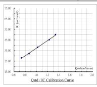
Calibration curve requirements: (A). r > 0.990; (B). At least 3 Qstd numbers are in the TSP range (1.1 - 1.7 m3 / min).
