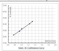
$Calibration \ curve \ requirements: \quad (A). \ \ r > 0.990 \ ; \ \ (B). \ \ At \ least \ 3 \ Qstd \ numbers \ are in the \ TSP \ range \ (\ 1.1 - 1.7 \ m3 \ / \ min \ ).$
