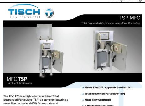
consistent particulate sampling. The mass flow controller adjust the motor speed as the filter media collects particulate to maintain a constant flow rate throughout the entire sample duration. The system utilizes a stainless steel filter holder for use with standard 8" x 10" filter paper. The anodized aluminum shelter and robust electrical components allow the system to operate a continuous 24 hour sample.
