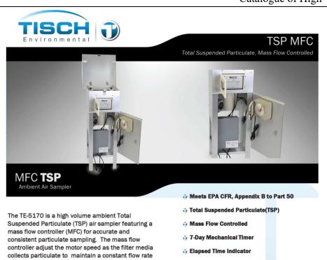
consistent particulate sampling. The mass flow controller adjust the motor speed as the filter media collects particulate to maintain a constant flow rate throughout the entire sample duration. The system utilizes a stainless steel filter holder for use with standard 8" x 10" filter paper. The anodized aluminum shelter and robust electrical components allow the system to operate a continuous 24 hour sample.
