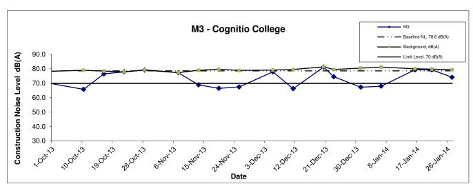
Remark: The measurement of Background Noise at M3 was started from 9 September 2013 for compliance checking of Noise Action/Limit Level.
