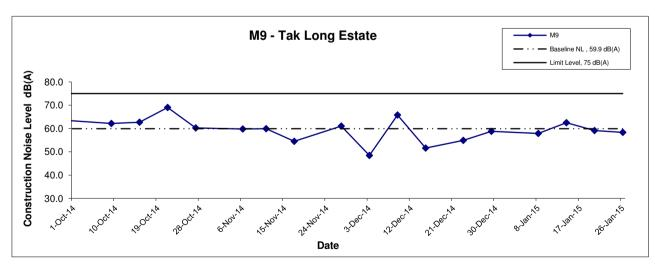
Remarks: The construction noise levels in the Tables in Appendix G were adopted for plotting the graphs The Limit level for M3 and M4 are 65dB(A) during the examination period
