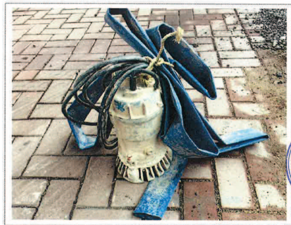
CNP 283 Water pump, submersible (electric)
