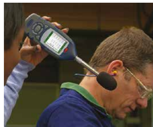
Small and lightweight with a bright colour display, the 63x Series makes workplace noise measurements easy
