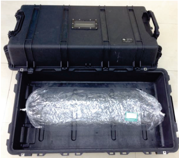
Figure 1a: Sampling Bag & Air-tightened Sampler
