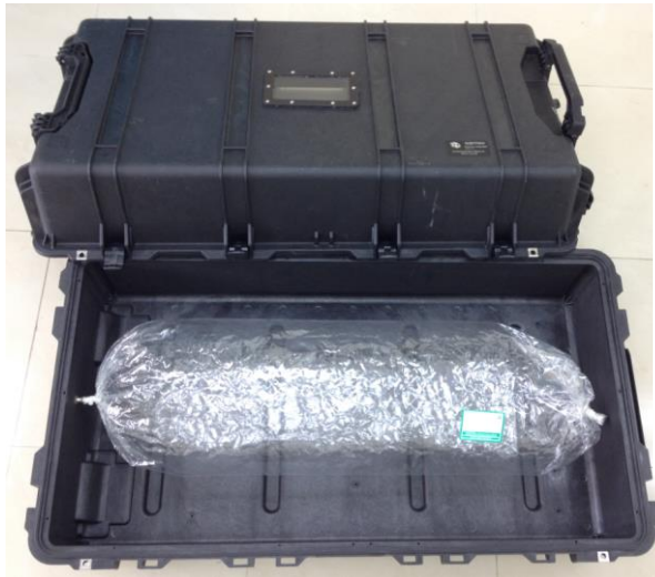
Figure 1a: Sampling Bag & Air-tightened Sampler
