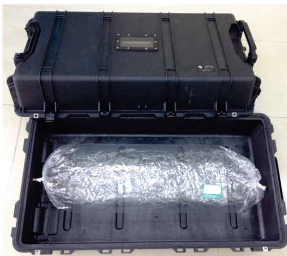
Figure 1a: Sampling Bag & Air-tightened Sampler
