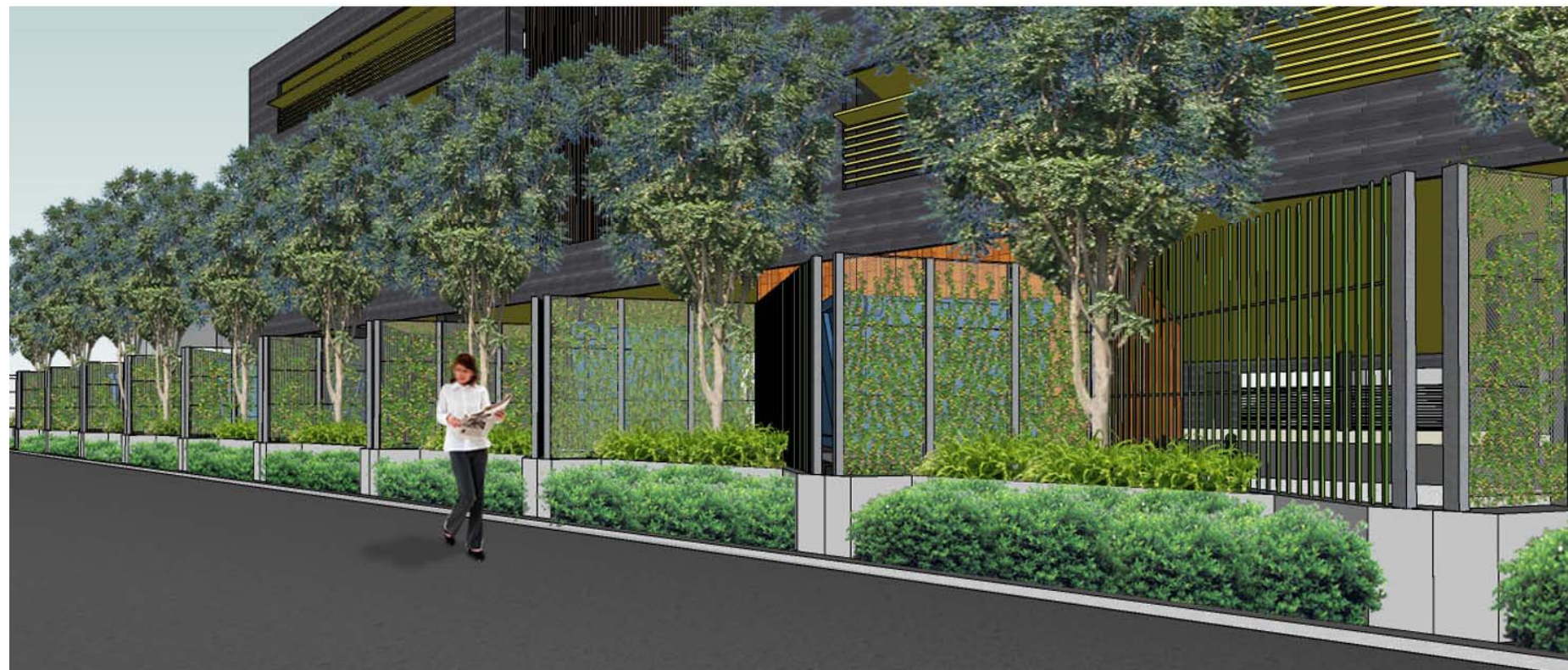
Figure 6 – Type 1 Vertical Greening System (Ground Floor)
