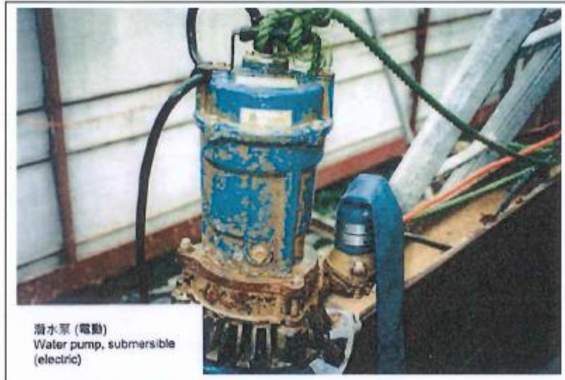
CNP 283 Water pump, submersible (electric) 潛水泵 (電動)
