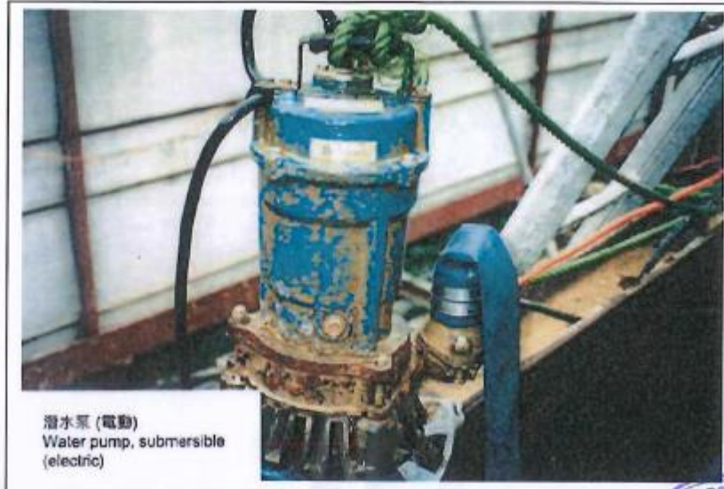
CNP 283 Water pump, submersible (electric) 潛水泵 (電動)
