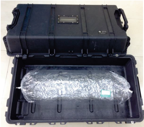
Figure 1a: Sampling Bag & Air-tightened Sampler
