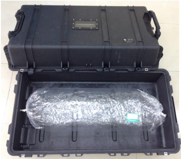
Figure 1a: Sampling Bag & Air-tightened Sampler
