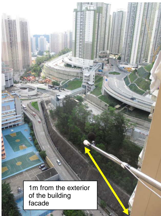
Figure 2 Equipment set-up at Tat Chui House
