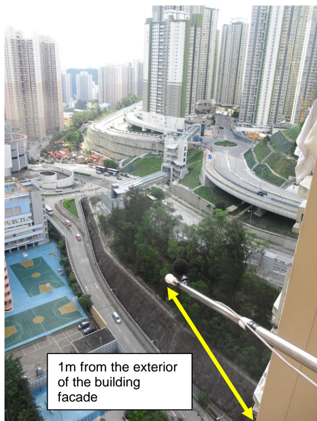
Figure 2 Equipment set-up at Tat Chui House
