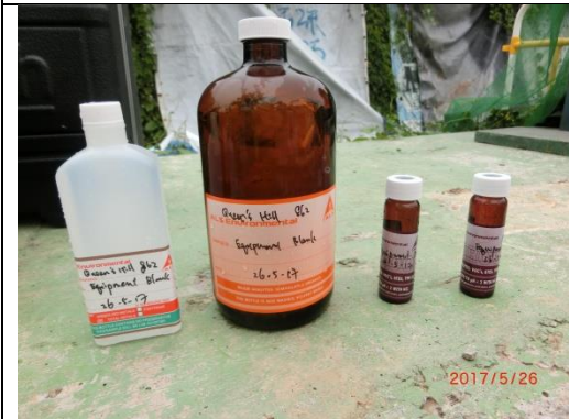
Equipment Blank for Groundwater Sample
