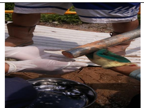
Collect soil sample with cleaned stainless steel equipment
