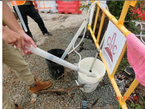
Cleaning of equipment before groundwater well purging with phosphate-free detergent (Decon® 90)
