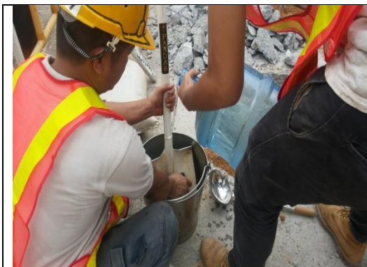
Cleaning of equipment with phosphate-free detergent (Decon® 90)
