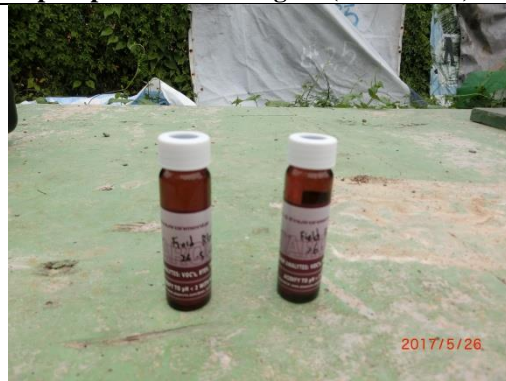
Field Blank for Groundwater Sample
