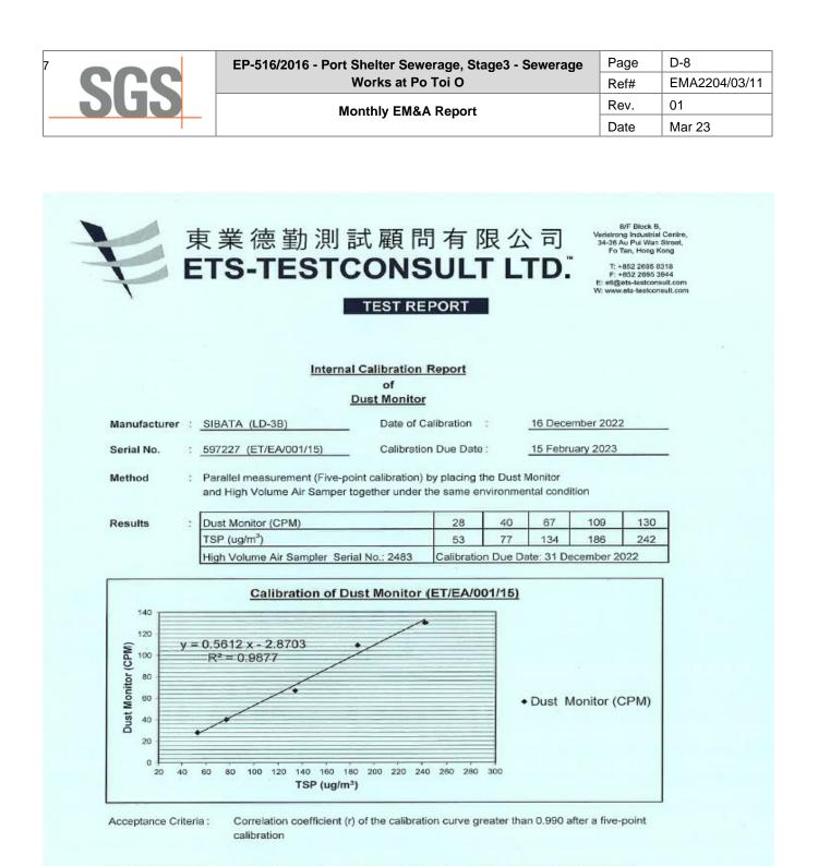
The Dust Trak Monitor complies \* / does not comply \* with the internal calibration procedures and is deemed acceptable \*/ unacceptable \* for use.
