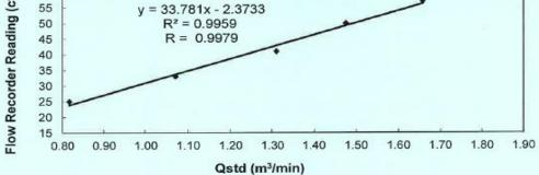
Acceptance Criteria : Correlation coefficient (r) of the calibration curve greater than 0.990 after a 5-point calibration
