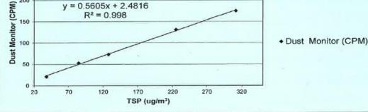
Acceptance Criteria : Correlation coefficient (r) of the calibration curve greater than 0.990 after five-point calibration.
