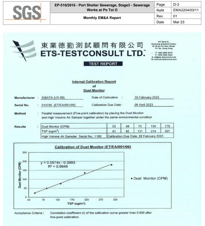
The Dust Trak Monitor complies \* / does not comply \* with the internal calibration procedures and is deemed acceptable \*/ unacceptable \* for use.
