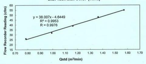
Acceptance Criteria: Correlation coefficient (r) of the calibration curve greater than 0.990 after a 5-point calibration.
