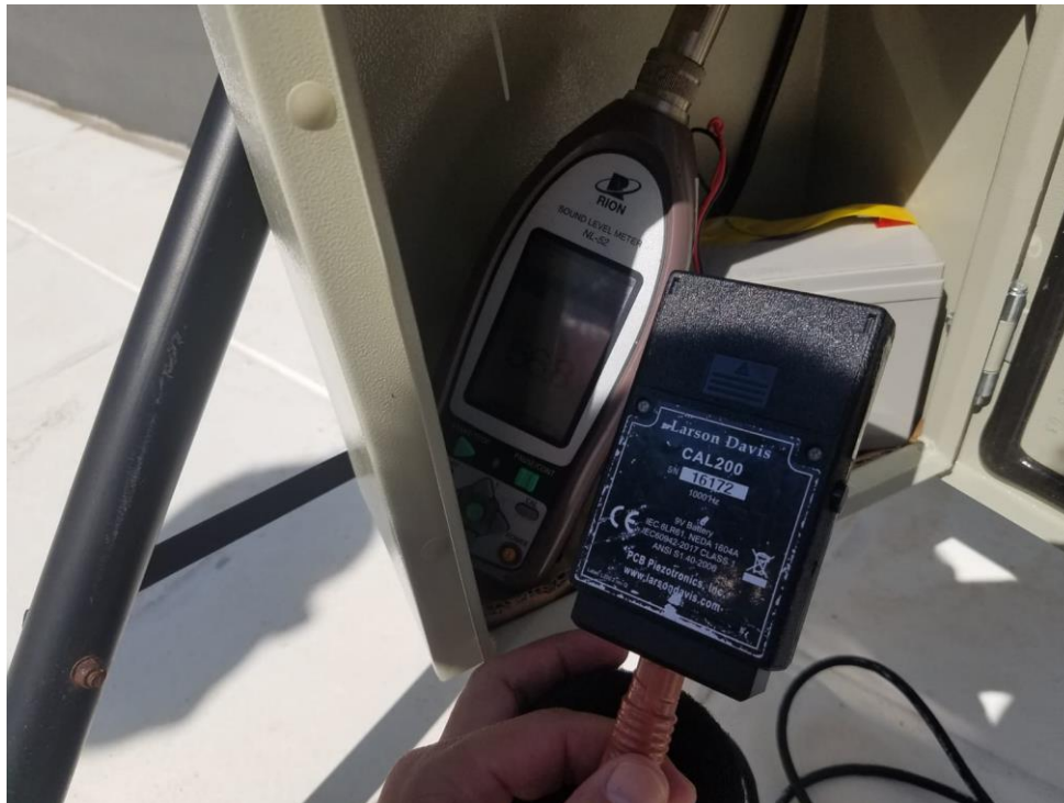
Noise monitoring equipment at NMS-CA-9
