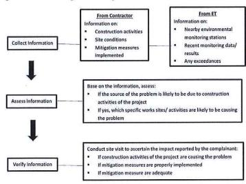
Figure 5.1: Investigation Stage Process flow Chart
