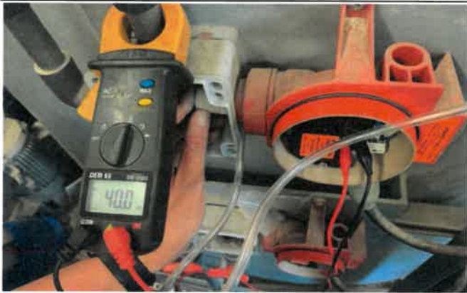
5ppm H2S Calibration for Outlet H2S Sensor
