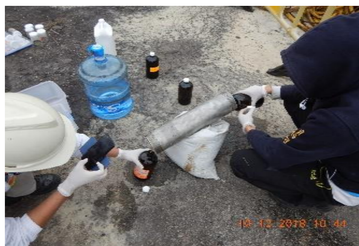
Collecting Equipment Blank for Soil Sampling
