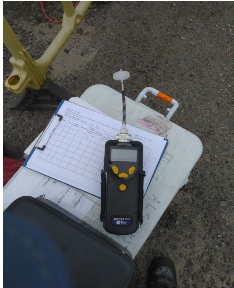
Measurement of Background VOC Concentration (Below: Close-up view)
