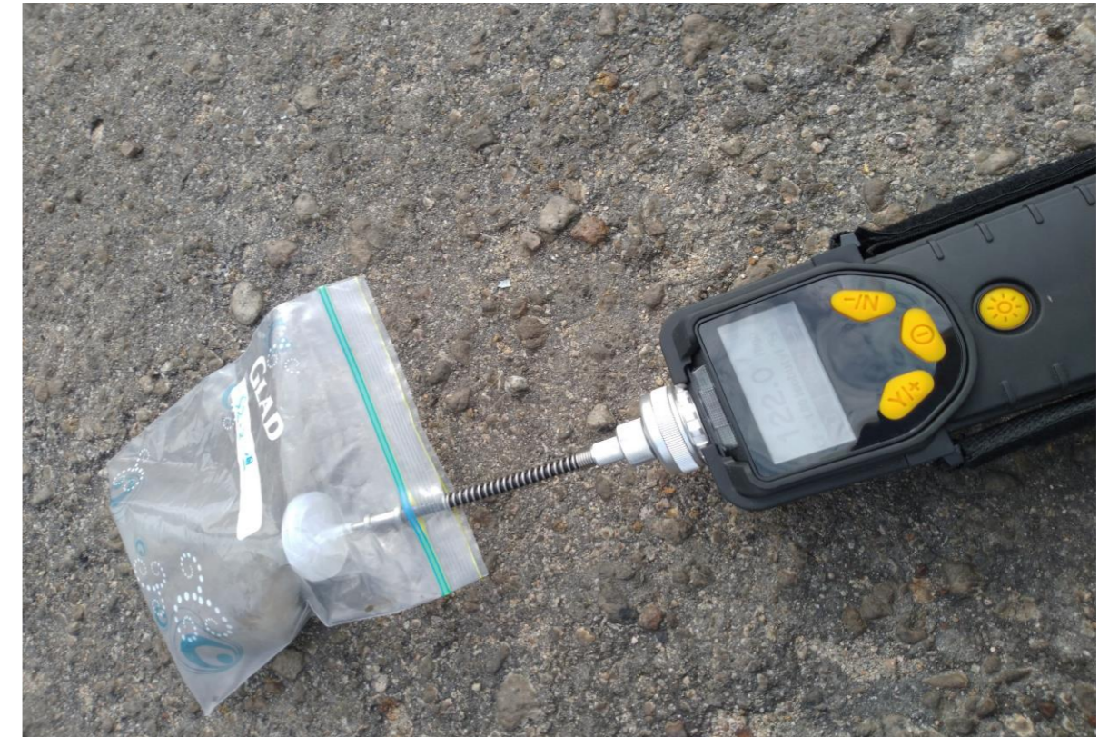
Put the probe of the VOC Sampler to the Bag for Measurement
