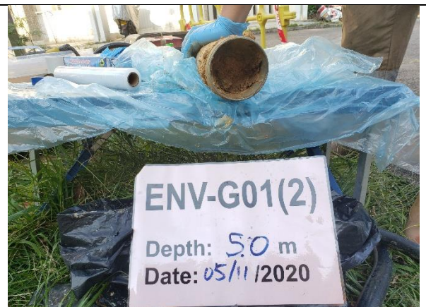
Photo 12 – Undisturbed soil sample collected at 5.0m at ENV-G01(2). No smell and NAPL were observed.
