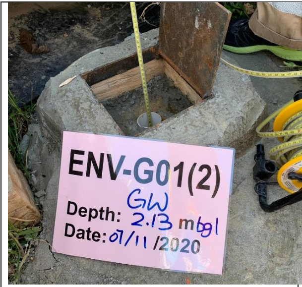
Photo 13 – Groundwater Monitoring Well at 2.13m at ENV-G01(2)
