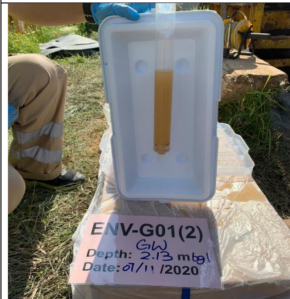
Photo 15 – Groundwater Sampling at 2.13m at ENV-G01(2). No smell and NAPL were observed.
