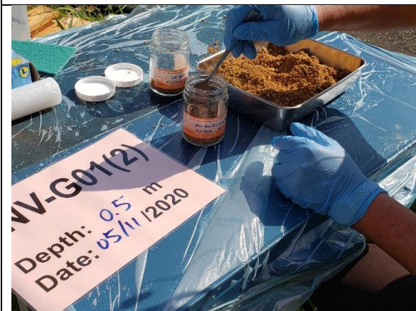
Photo 7 – Sampling of ENV-G01 (2) at 0.5m depth. No NAPL was observed.
