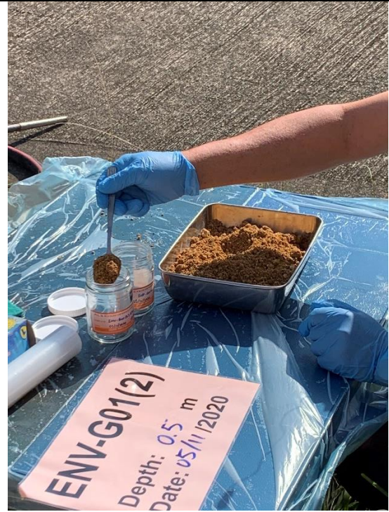
Photo 6 – Sampling of ENV-G01 (2) at 0.5m depth. No NAPL was observed.
