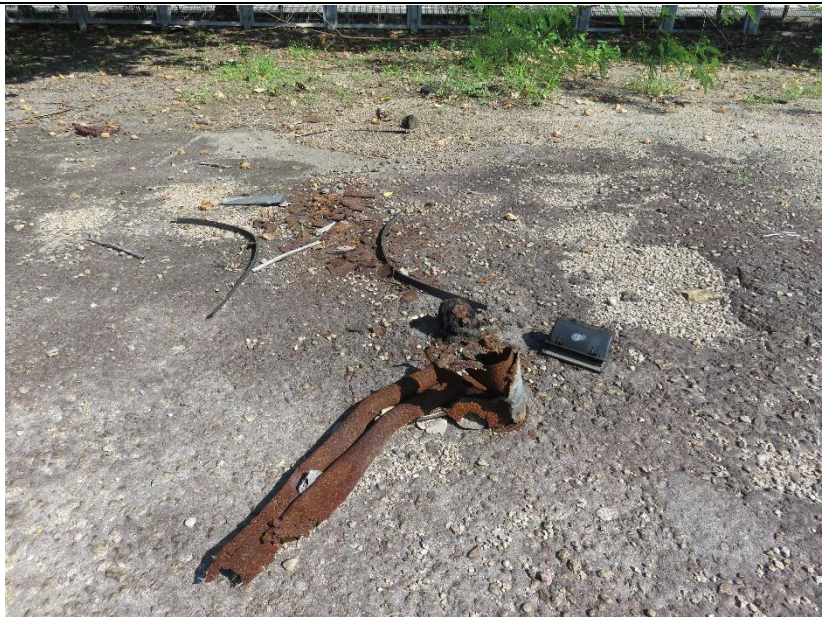
Broken Exhaust Pipe
