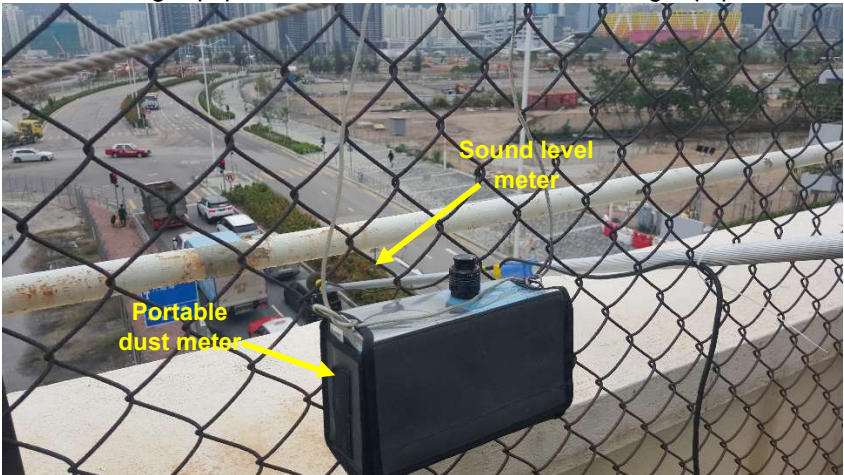
Air monitoring equipment at AMS1 and noise monitoring equipment at NMS1
