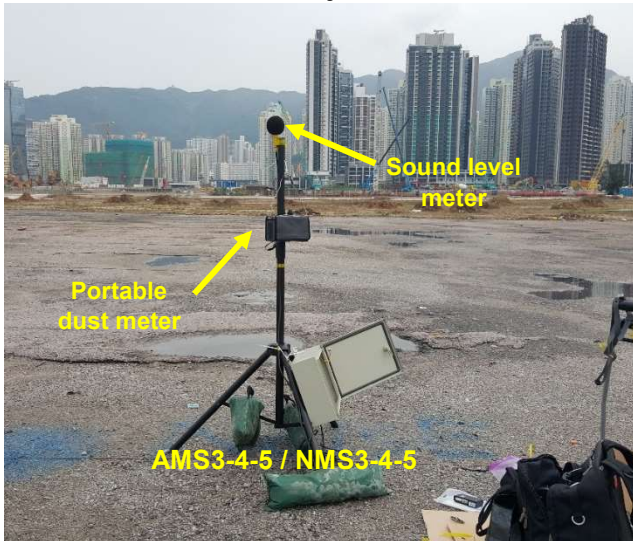
Air monitoring equipment at AMS3-4-5 and noise monitoring equipment at NMS3-4-5
