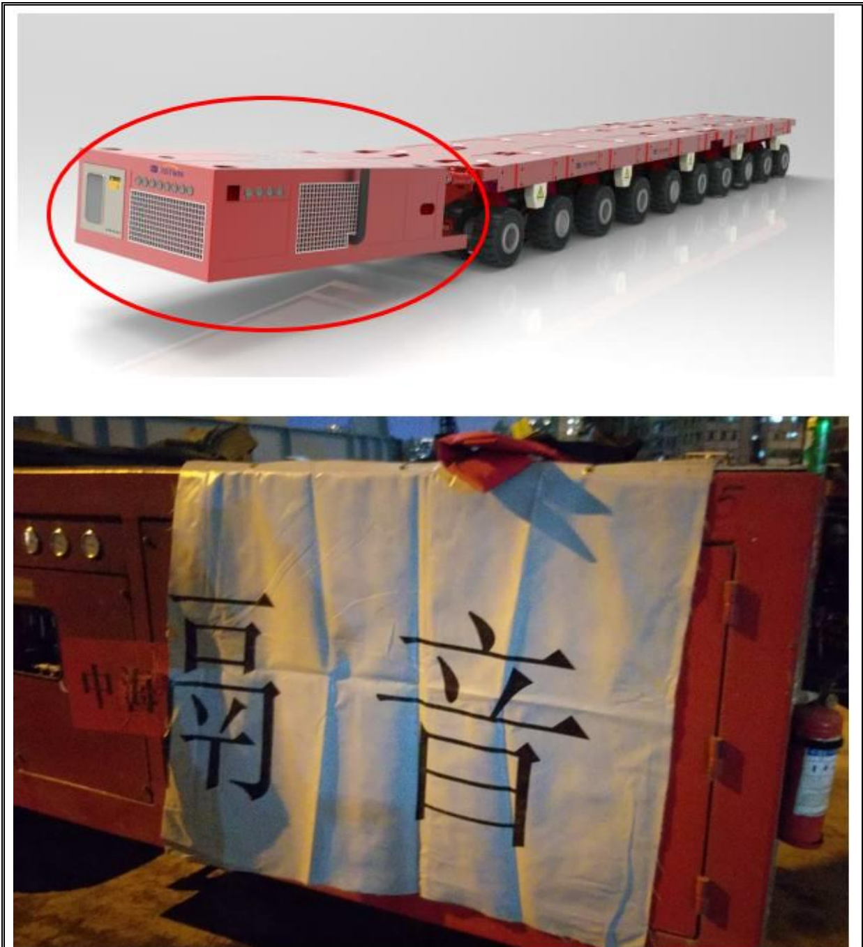
Photos 2a and 2b: Noise insulating fabric implemented on moving trailer according to the CNP requirement. (12 November 2021)
