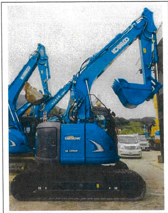
Excavator, tracked, with Quality Powered Mechanical Equipment Label showing a Sound Power Level \leq 92 dB(A) 挖土機，履帶式，備有優質機動設備標籤顯示聲功率級 \leq 92 分貝(A)
