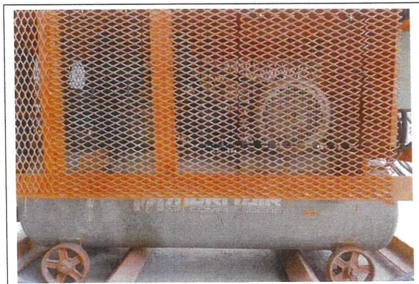
Air compressor, with Noise Emission Label showing a Sound Power Level \leq 97 dB(A)
