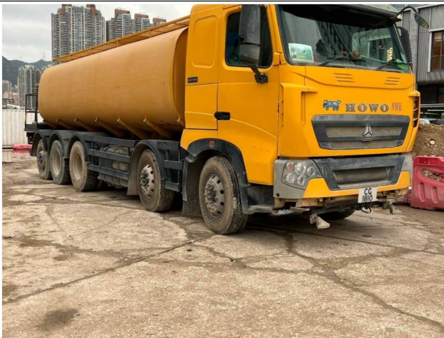
Photo 3: Water spraying truck has been provided at the meantime to minimize the dust nuisance at the concerned area.
