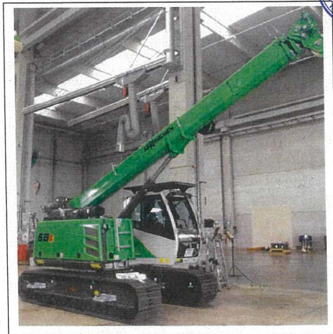
Crane, mobile (diesel), with Quality Powered Mechanical Equipment Label showing a Sound Power Level \leq 102 dB(A)
