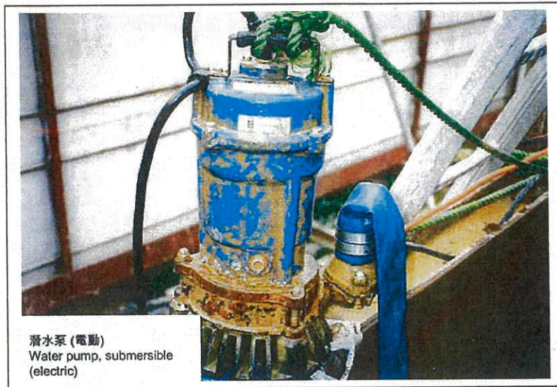
CNP 283 Water pump, submersible (electric) 潛水泵 (電動)
