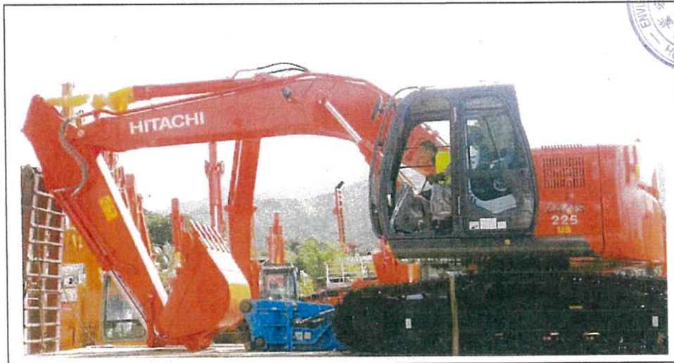
Excavator, tracked, with Quality Powered Mechanical Equipment Label showing a Sound Power Level \leq 103 dB(A) 挖土機，履帶式，備有優質機動設備標籤顯示聲功率級 \leq 103 分貝 (A)
