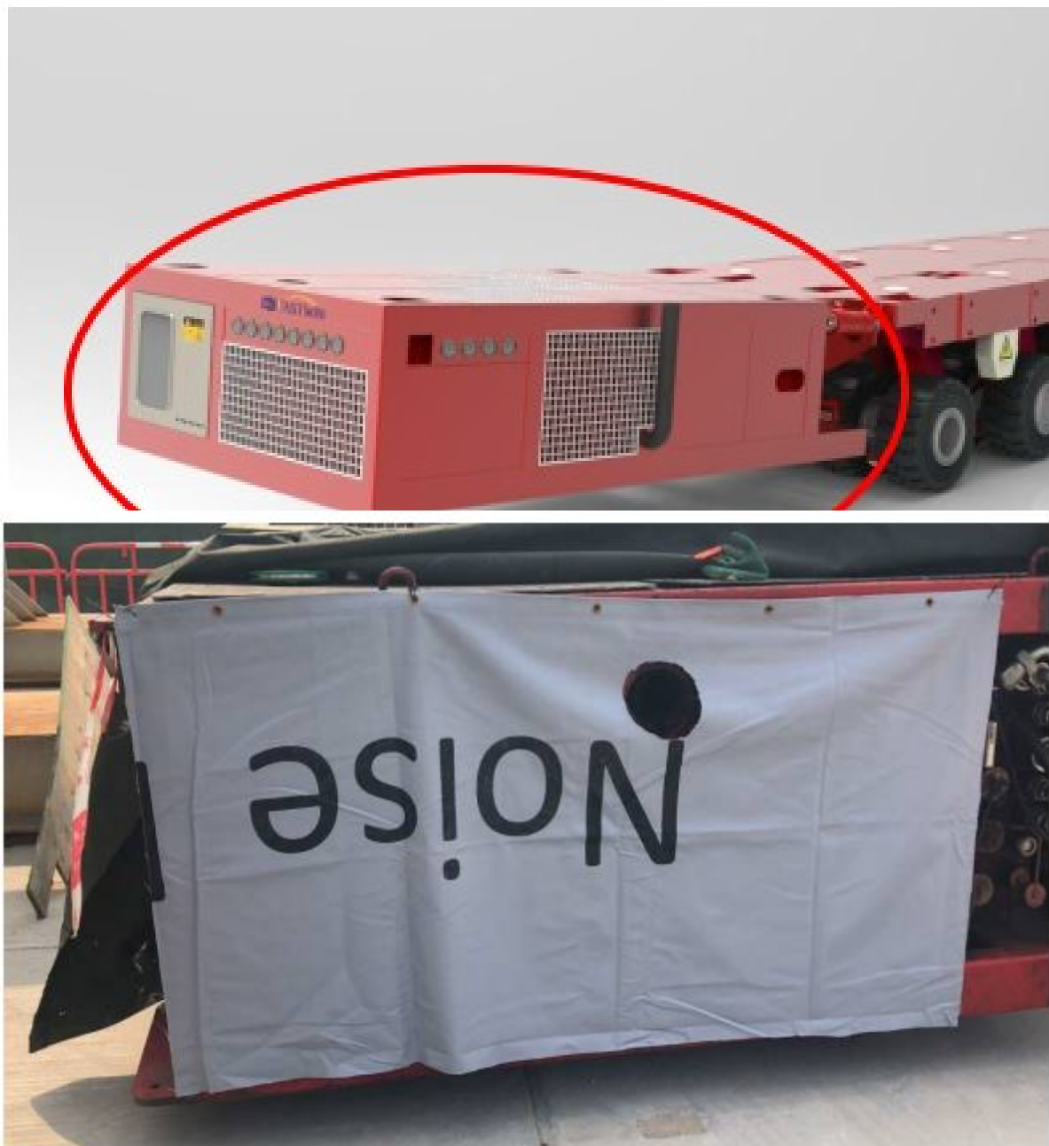
Photos 2a and 2b: Noise insulating fabric implemented on moving trailer according to the CNP requirement.
