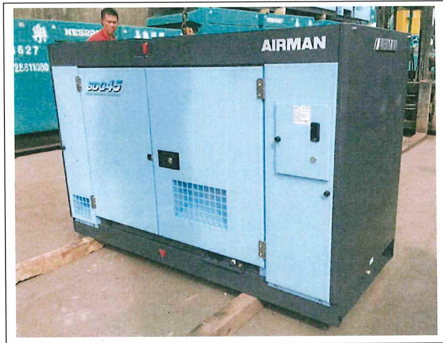
Generator, with Quality Powered Mechanical Equipment Label showing a Sound Power Level of \leq 87 dB(A)
