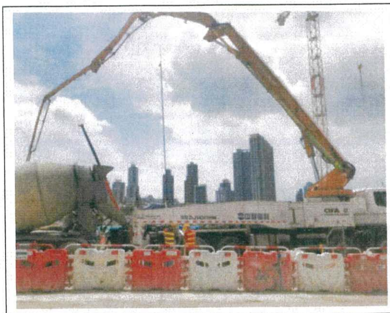
Concrete pump, lorry mounted (Model No. 56X-6RZ / Serial No. ZLJ5430THBK) 混凝土泵，裝在貨車上 (型號 56X-6RZ / 序號 ZLJ5430THBK)
