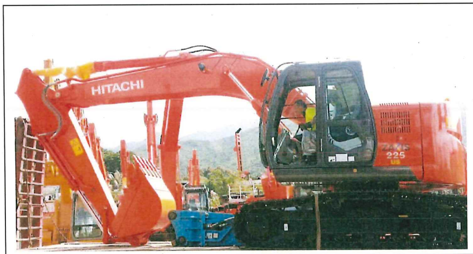
Excavator, tracked, with Quality Powered Mechanical Equipment Label showing a Sound Power Level of \leq 100 dB(A)
