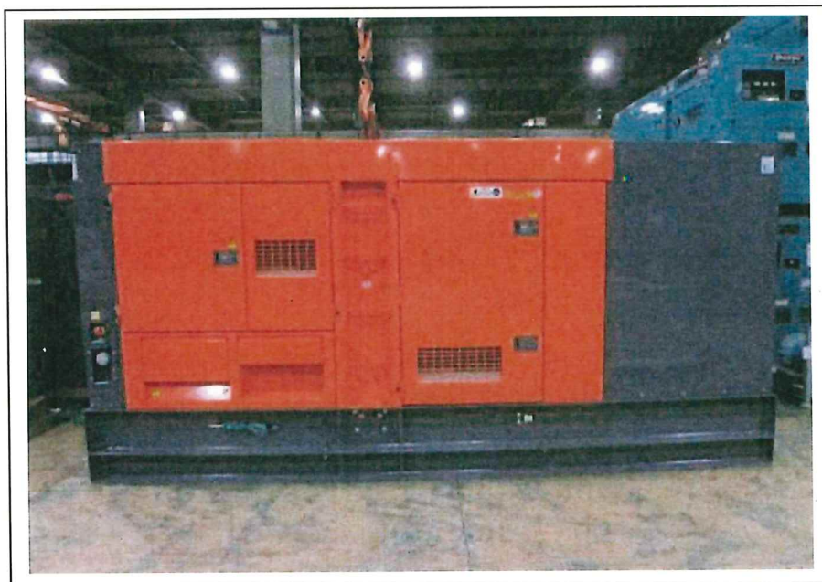
Generator, with Quality Powered Mechanical Equipment Label showing a Sound Power Level of \leq 97 dB(A)
