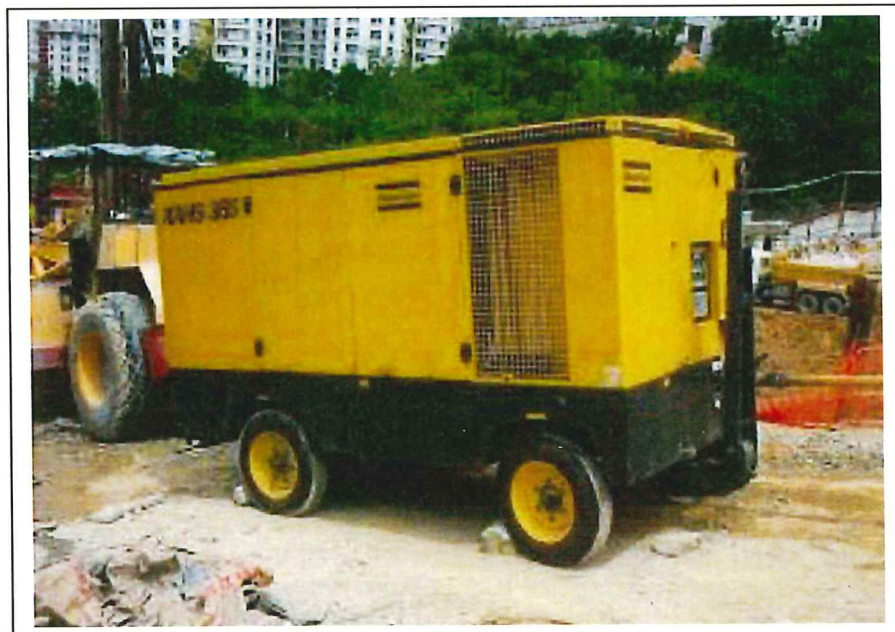
Air compressor, with Noise Emission Label showing a Sound Power Level of \leq 102 dB(A)
