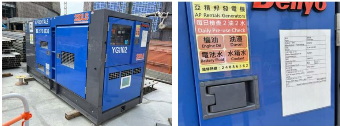
Photo 2a and 2b: Power Mechanical Equipment with Quality Power Mechanical Equipment (QPME) labels were used at site to lower the noise nuisance to the nearby residents.
