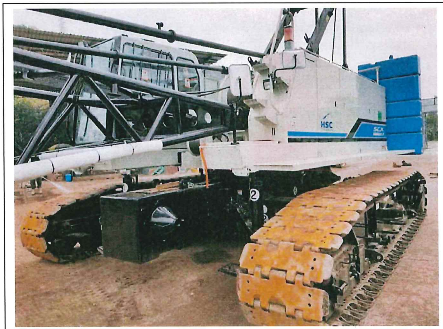
Crane, mobile (diesel), with Quality Powered Mechanical Equipment Label showing a Sound Power Level of \leq 103 dB(A)
