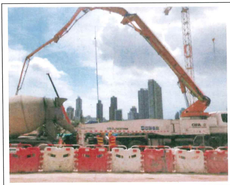
Concrete pump, lorry mounted (Model No. 56X-6RZ / Serial No. ZLJ5430THBK) 混凝土泵，裝在貨車上 (型號 56X-6RZ / 序號 ZLJ5430THBK)
