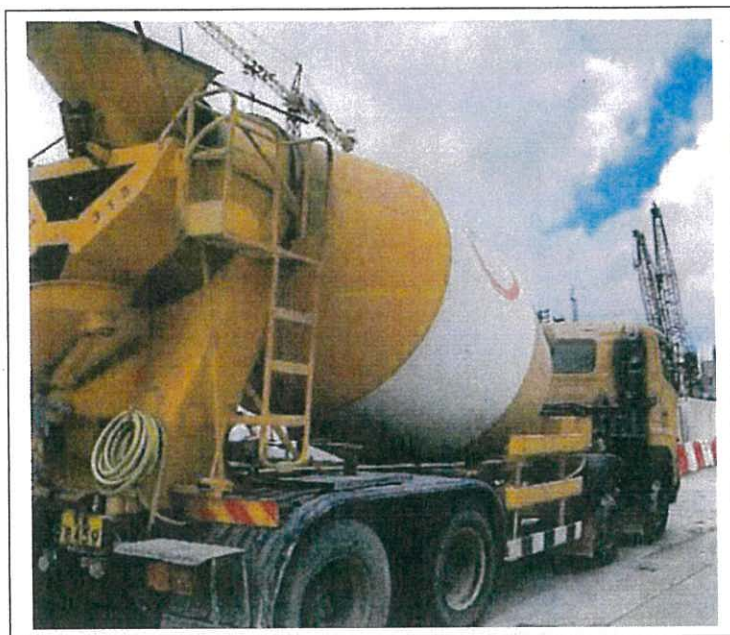
Concrete lorry mixer (Vehicle No. KK8459)
