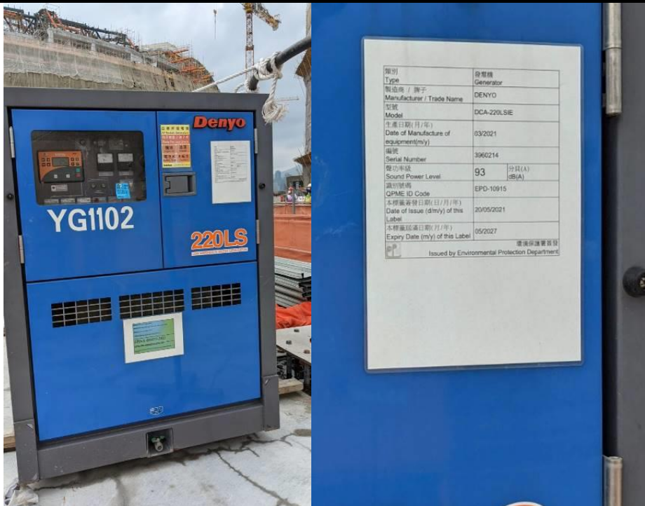
Photos 2a and 2b: Power Mechanical Equipment with Quality Power Mechanical Equipment (QPME) labels were used at site to lower the noise nuisance to the nearby residents
