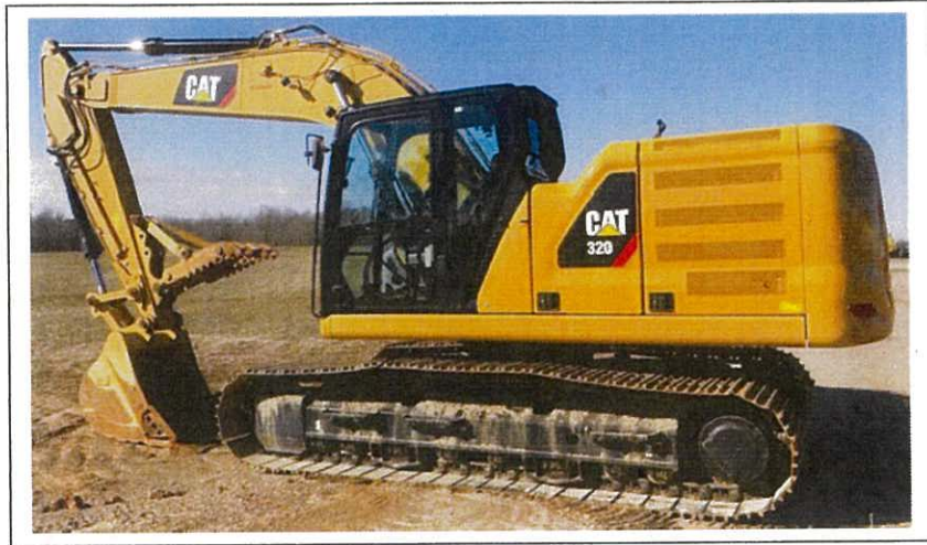
Excavator, tracked, with Quality Powered Mechanical Equipment Label showing a Sound Power Level \leq 98 dB(A) 挖土機，履帶式，備有優質機動設備標籤顯示聲功率級 \leq 98 分貝 (A)
