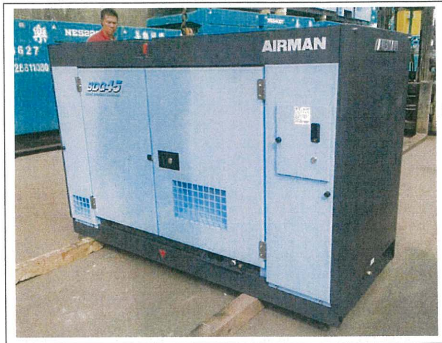
Generator, with Quality Powered Mechanical Equipment Label showing a Sound Power Level \leq 87 dB(A)
