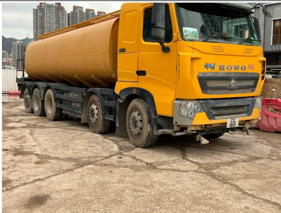
Photo 3: Water spraying truck has been provided at the meantime to minimize the dust nuisance at the concerned area.
