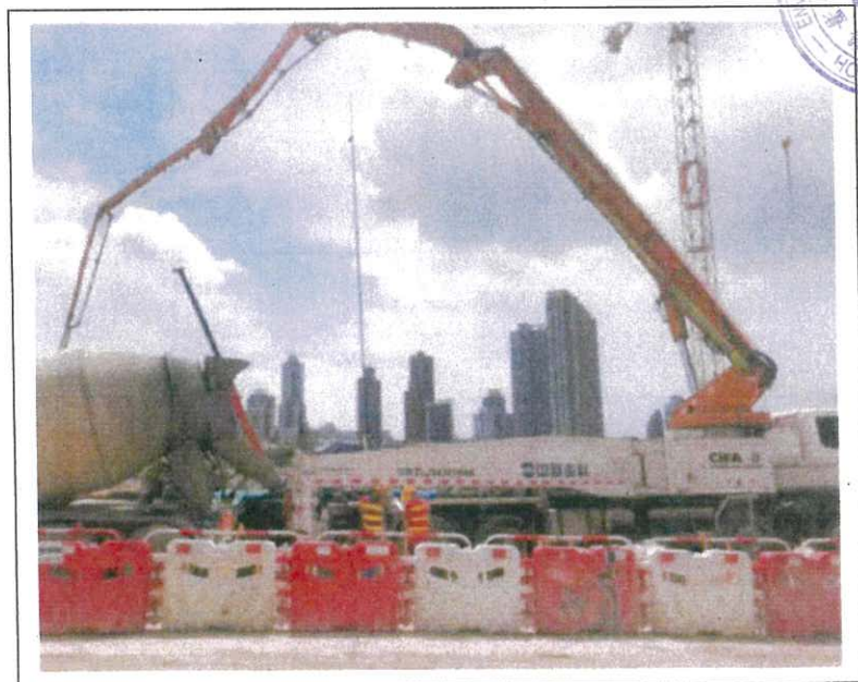
Concrete pump, lorry mounted (Model No. 56X-6RZ / Serial No.
