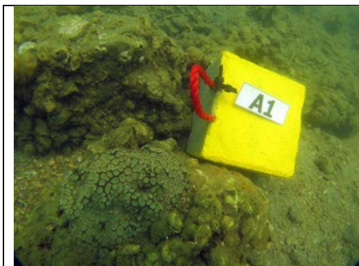
Photo 5.1 Concrete block in bright color can be used for coral tagging.
