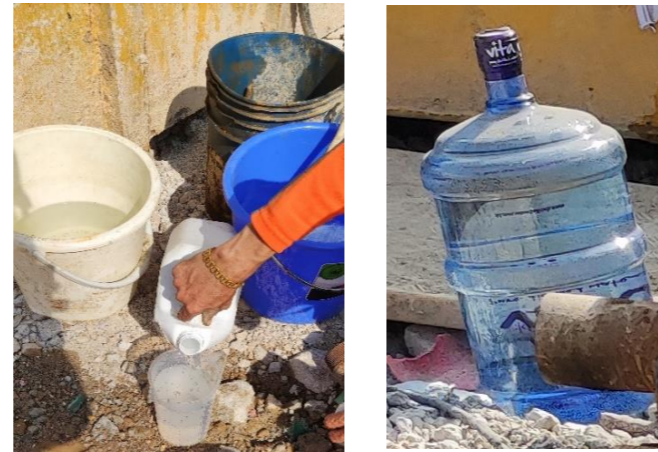
Cleaning with lab-grade detergent and distilled Water
