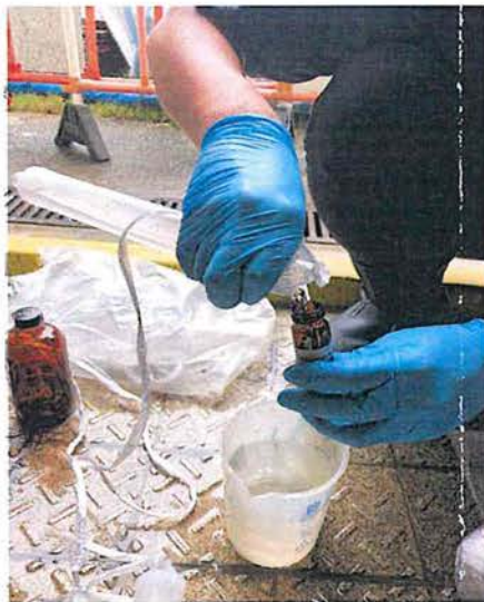
Collecting Equipment Blank for GW Sampling
