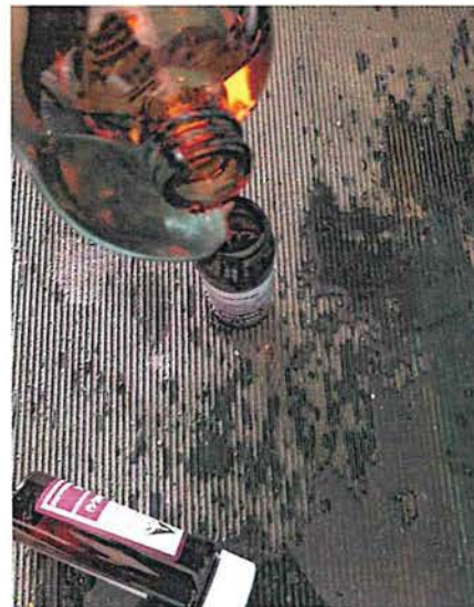
Collecting Equipment Blank for Soil Sampling
