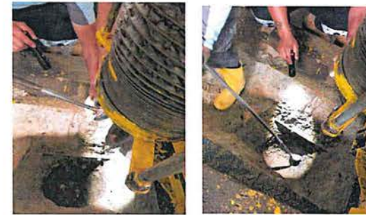
Collecting Soil Samples at 0.5m bgl
