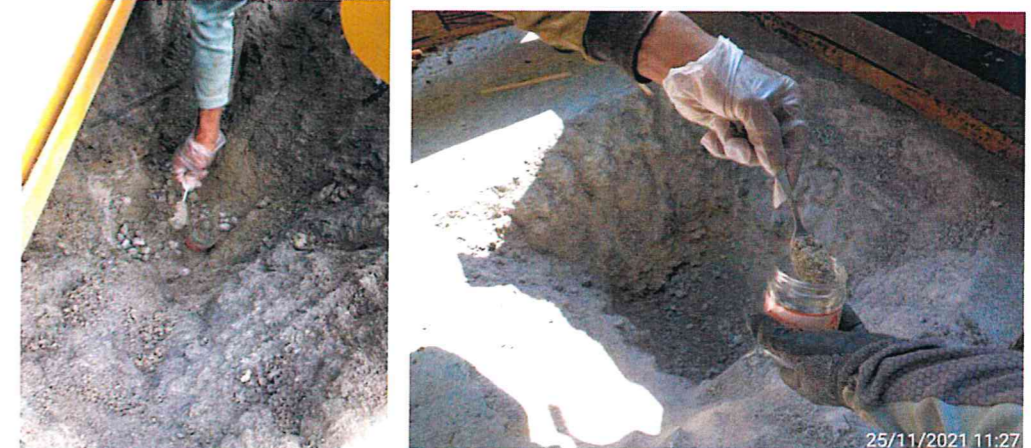
Collecting Soil Samples at 0.5m bgl
