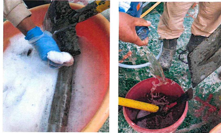
Cleaning with lab-grade detergent and distilled Water
