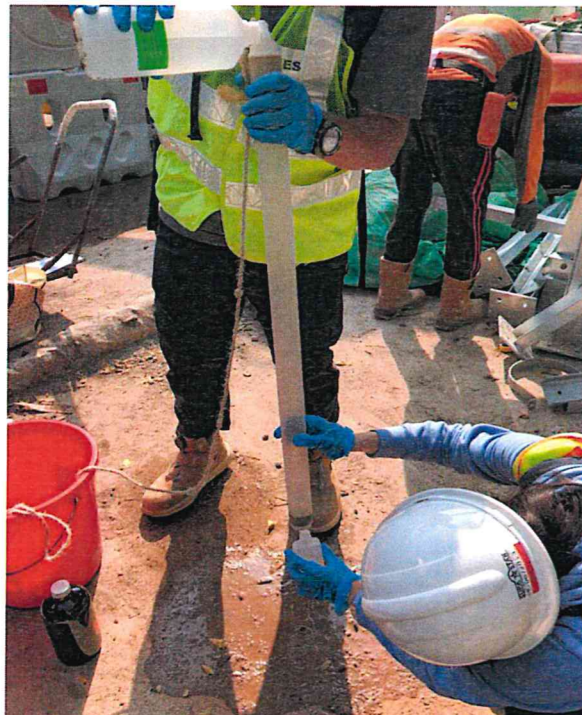
Collecting Equipment Blank for GW Sampling
