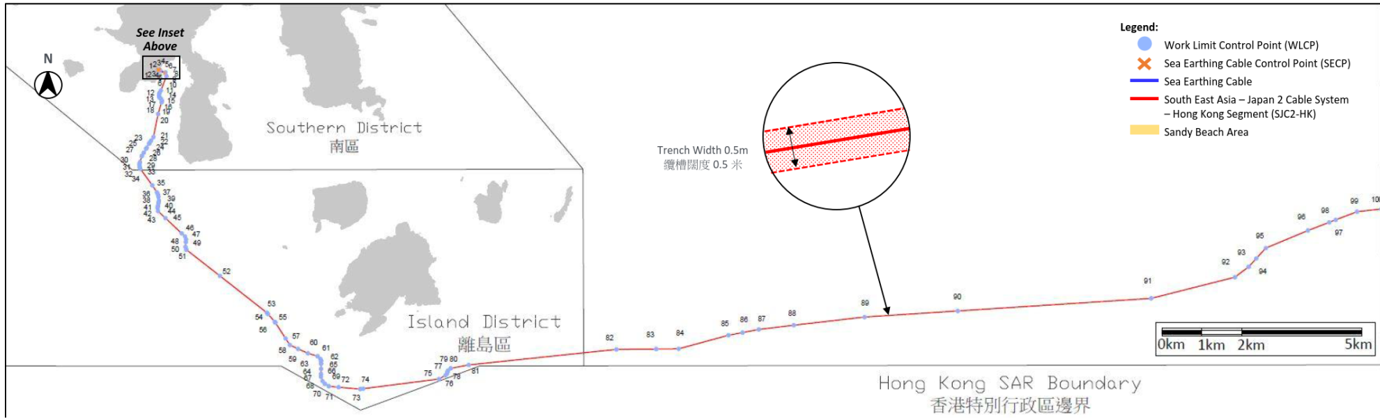
Figure 1.1 Alignment of SJC2-HK Cable System within Hong Kong (Source: Figure 1.3 of the Project Profile)
